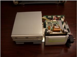
Step 3 - Removing the power supply
