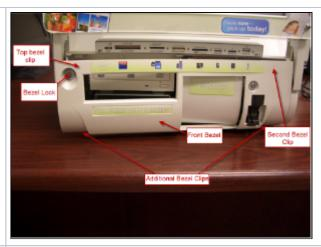
Completely remove the front bezel and place it somewhere safe. Once the bezel is removed, the Optical Drive and Receipt Printer tray will be exposed.
