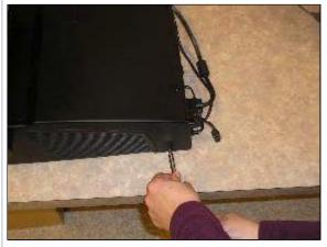
There is a fifth screw located behind the monitor and underneath the receipt panel, make sure to unscrew that as well.
