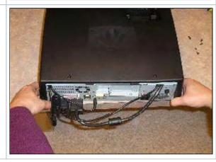
• Remove the cover plate. Unscrew the side-mounted screws from the front panel. • Pull to remove the front panel.
