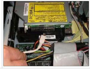
• To replace the CD/DVD drive, get a small screwdriver and unscrew it from the bracket.
