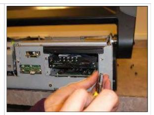
• Unplug the IDE cable and power supplies connected to the CD/DVD drive.
