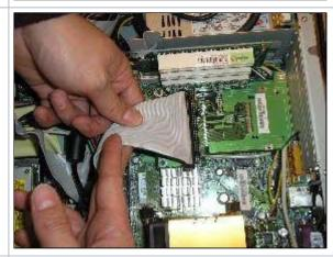
Unplug the USB connected to the inside of the card reader. The card reader should slide out of the front of the unit.
