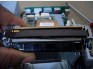
Step 4 - Remove Rollers from the back of the front panel (only if necessary)
