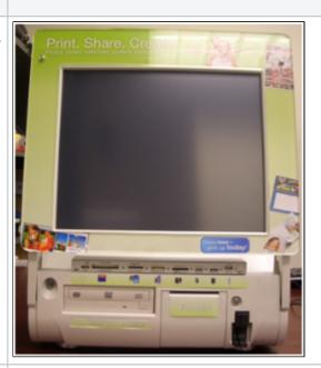
Insert the larger key of the two sets provided into the lock located on the top, left panel of the kiosk's front bezel. Set the lock to the "on" position.
