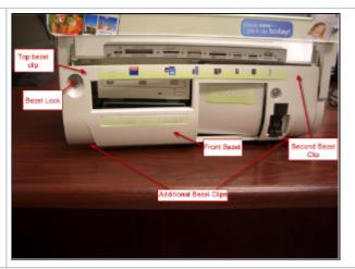
Completely remove the front bezel and place it somewhere safe. Once the bezel is removed, the Optical Drive and Receipt Printer tray will be exposed.
